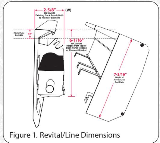
Figure 1. Revital/Line Dimensions
