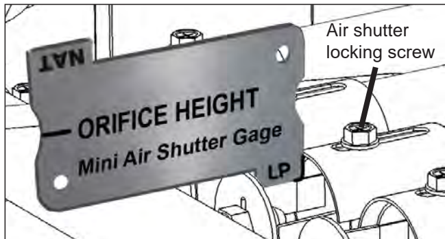
Figure 39. The Mini-Gauge (included with the installation kit) for Orifice Adjustment
